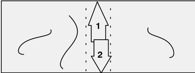
**Figure 4. Squeegeeing the Center of a Large Graphic**
